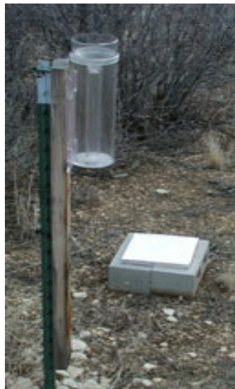
Mounted rain gauge and hail pad
