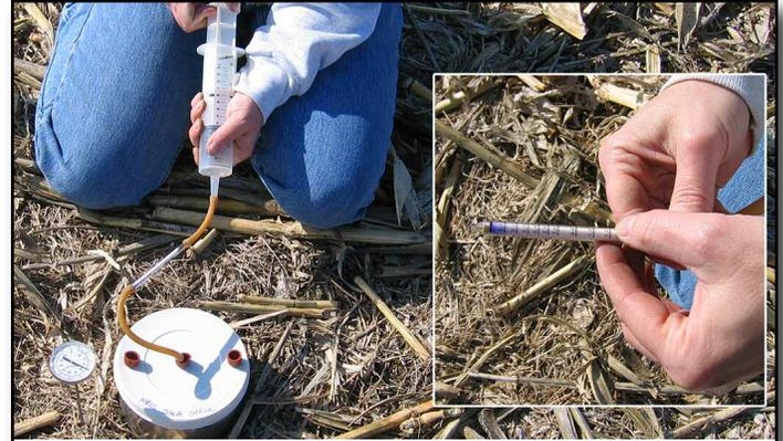
*Figure 1. Draeger-Tubes® are used to measure CO<sub>2</sub> released from the soil surface as an indicator of decomposition and soil respiration.*
